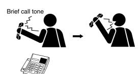
**Step 3.** To terminate the conversation, replace the handset or press the [C] key.
